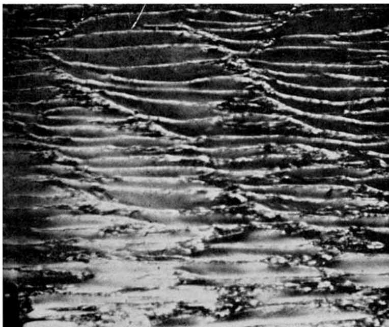
Fig. 9. Details of fast crack growth region shown in Fig. 8 (27 \times ).
